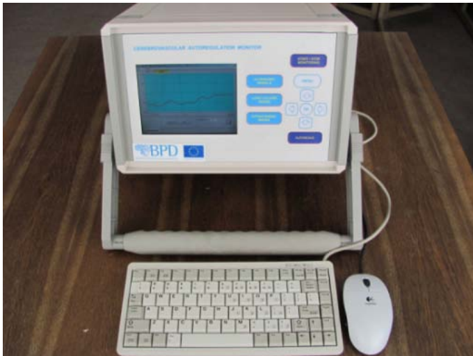
Figure 1: Non-invasive monitor for continuous real time monitoring of cerebrovascular autoregulation
