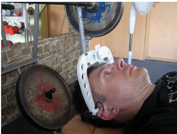
Figure 2: The mechanical frame mounted on the sportsman head in order to fix ultrasonic transducers for transmitting ultrasonic signal through brain parenchyma
